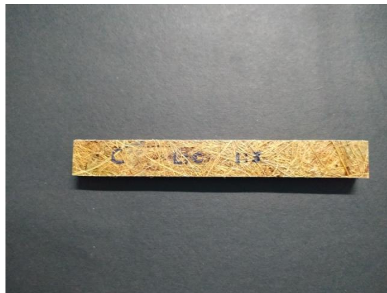
Fig. 5 Specimen for Flexural test.
