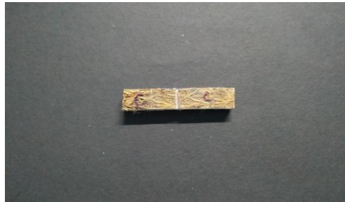
Fig 6. Specimen for Charpy Impact test.
